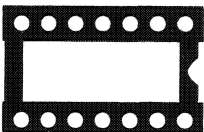
IC-socket with marker notch
